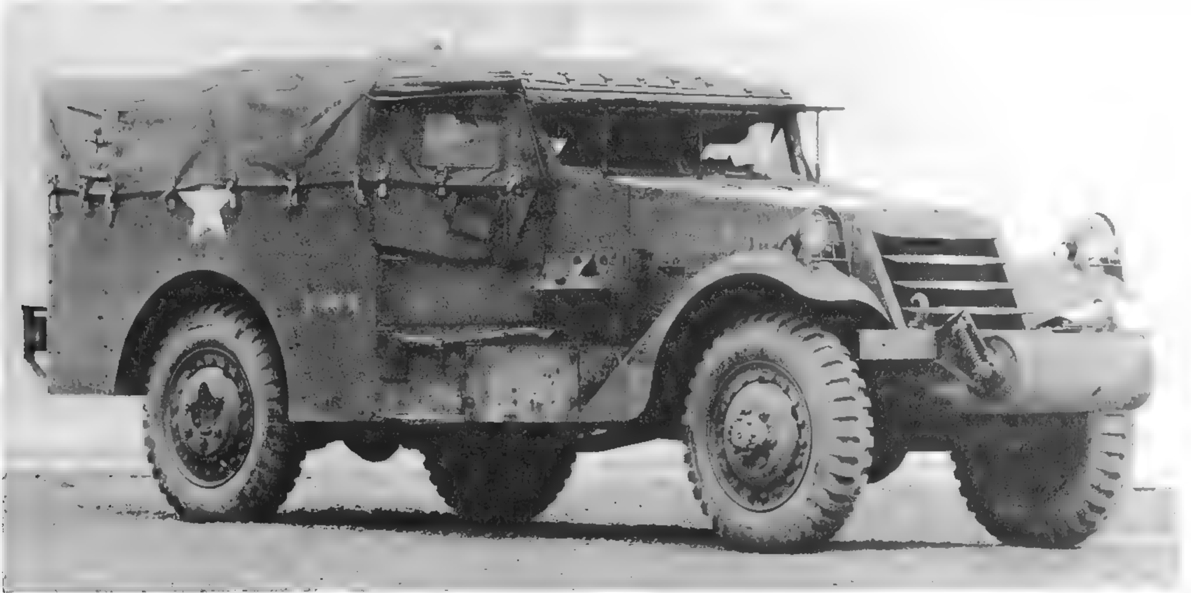
The M3A1 was provided with a canvas covering, shown in this April 1944 Studebaker Proving Ground photo. Gone are the spotlights, externally stored collapsible canvas bucket, crossed sabers, and greenhouse-type windshield of the early models. Instead, there are liquid container carriers and removable windshield glasses. (U.S. Army photo)
